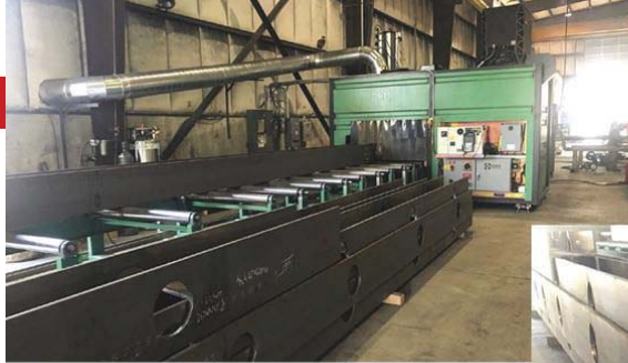
The SteelPRO system (above) can cut five or six angled holes through the flanges and webs of large I-beams, H-beams, tubing, angle, channel, flat bar, and bulb flats in 15 minutes, delivering squarer cut edges, markedly less angularity, and excellent surface finish on non-ferrous metals like aluminum and stainless steel. It can complete four beams in an hour, or 200 beams in 50 hours. This same work takes 1½ hours a piece by hand and requires 10-plus man-hours per beam, or 2,000 hours of labor.
