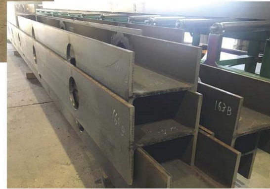
The SteelPRO system (above) can cut five or six angled holes through the flanges and webs of large I-beams, H-beams, tubing, angle, channel, flat bar, and bulb flats in 15 minutes, delivering squarer cut edges, markedly less angularity, and excellent surface finish on non-ferrous metals like aluminum and stainless steel. It can complete four beams in an hour, or 200 beams in 50 hours. This same work takes 1½ hours a piece by hand and requires 10-plus man-hours per beam, or 2,000 hours of labor.
